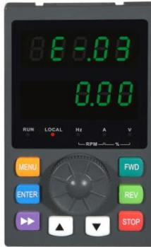
Fig. 4-5 Fault alarm display state
